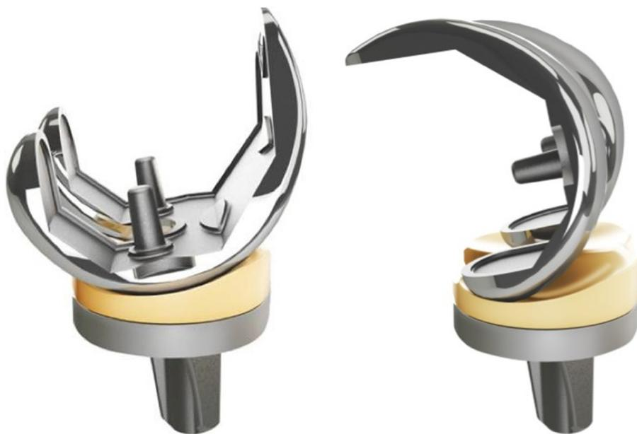
**Figure 1.** The ACL-substituting TKA design incorporates a lateral tibiofemoral compartment that is spherically conforming in extension, which becomes progressively more lax in flexion to allow the condyle to translate posteriorly.
